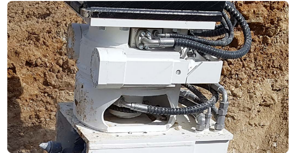
▲ A KRM 70 rotation unit extends the operating capabilities of a cutter attachment.
