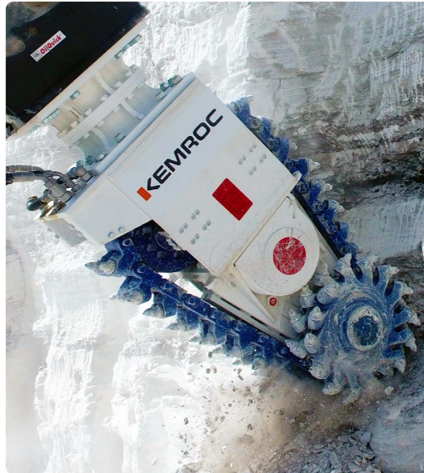
▲ Mining gypsum with an EK 100.
