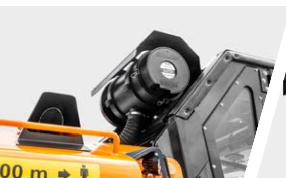
Cabin pressurization system
