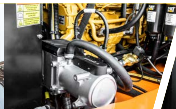
Pre-heating system for engine and hydraulic oil
