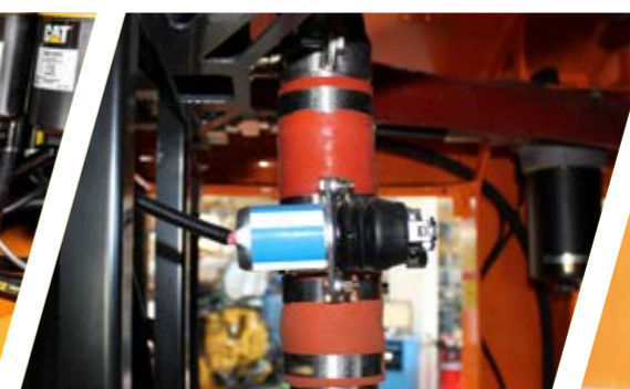
Air shut-off system
