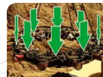
The particular structure allows the Pile Breaker to be positioned over the pile to be demolished.
